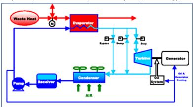
The ORC system will generate approximately 3,100 MWh annually from the waste heat from the car bottom furnaces and save approximately 13.8 million gallons of cooling water each year. In addition, because of the avoided electricity purchases, the estimated emissions savings resulting from reduced fossil fuel use by the local utility include the following:
