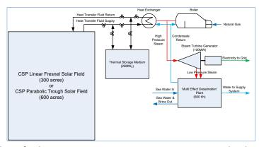
cycle and for mirror washing), so availability of adequate water is important. Water may also be produced using the available thermal energy from the solar field in an integrated combined heat and power desalination system.
